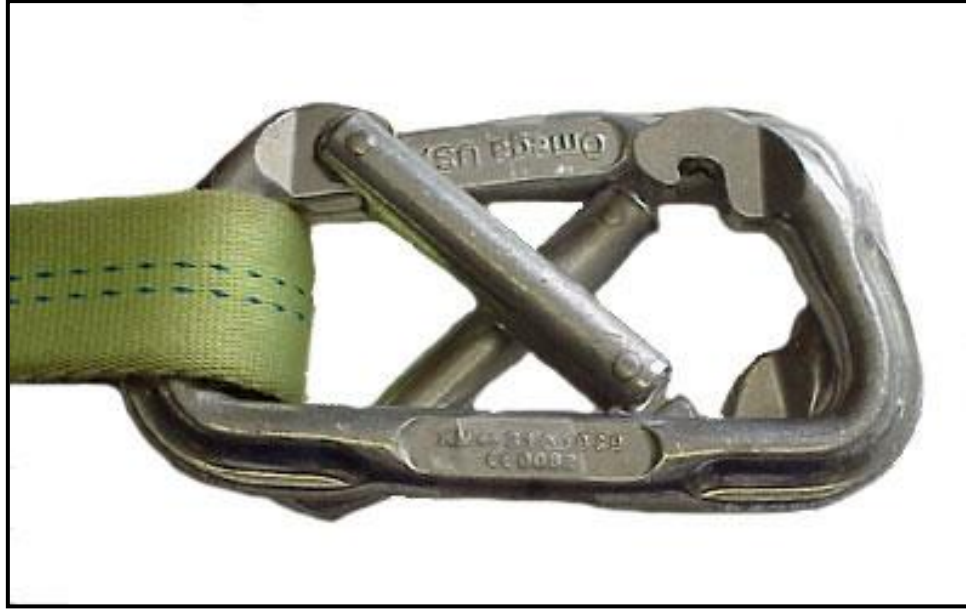
Figure 5-6. Correctly opposed carabiners.
